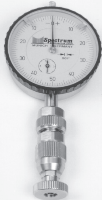
Type K: This gauge is available with a resolution of 0.01mm, or 0.001 inches.
